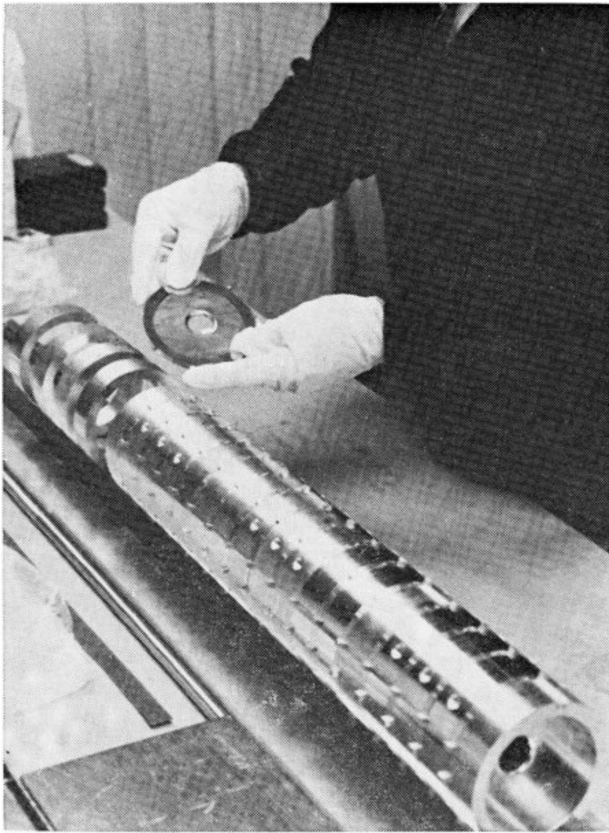
Figure 16. Assembly of a High Power Travelling Wave Accelerator Tube Prior to Brazing.
