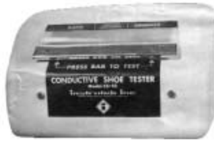
The CS-45 Conductive Shoe Tester was used to check safe shoe conductivity before entering an operating room.
